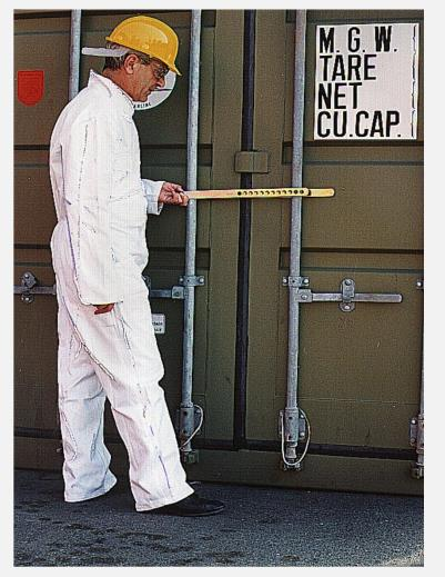
Barrier seal was created in the early '90s when it was discovered how to tamper with the openings of a container without touching the seal, but rather acting on the container handle.
