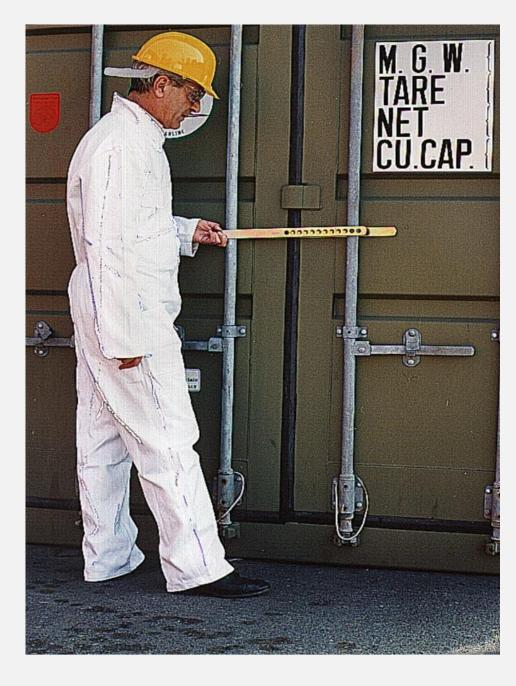
This security seal acts by clamping the two central barriers of the container and clearly blocking the doors opening.
