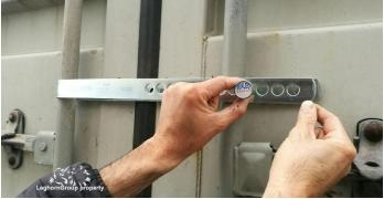
The two barriers should be blocked the closest possible in order to avoid any opening of the container.
