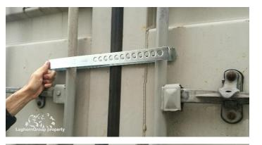
Insert the Forkseal between the two central barriers of the container, ensuring that the bend part of the barrier seal matches perfectly with the left barrier of the container.
