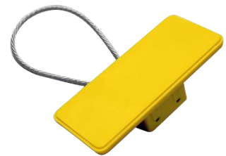
Art: RFID LOGISTIC CABLESEAL 3,5mm Cable seal Laser print Measures 3,5x200 mm ISO 17712:2013
