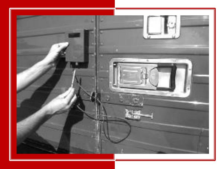
**eLOCK GOLD** is an advanced electronic reusable security lock, to control position and status of trucks and containers, either from fixed station or from mobile devices (smart phone and tablet).
