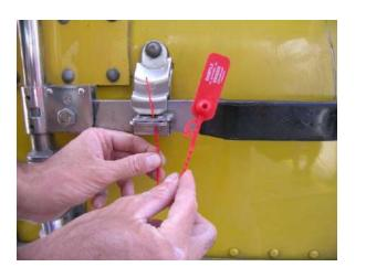
Insert the seal tail inside the door handle holes.
