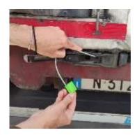
Insert the cable into the holes to be sealed.
