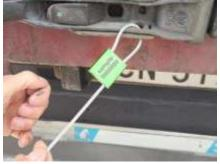
Insert the cable into the seal head hole and pull as much as possible to avoid any possibility the seal to be tampered with.
